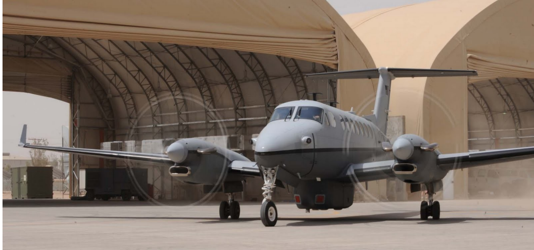
US Air Force Project Liberty King Air 350ER/MC-12 Airborne C4-ISR Aerial Surveillance Platform
